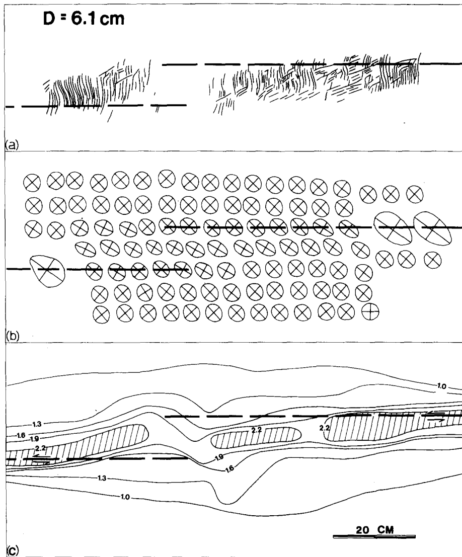
Fig. 2. Experimental results after displacement of 6.1 cm. Thick dashed lines represent position of underlying left-lateral strike-slip faults in basal plates. (a) Line drawing (traced from photograph) representing the fracture pattern consisting of Riedel shears, conjugate Riedel shears and slightly rotated conjugate Riedel shears. (b) Line drawing (traced from photograph) representing amount of strain sustained by clay. Similar line drawings are used to evaluate each stage illustrated in Figs. 3–6. (c) Contours of strain values calculated from each ellipse in (b). Hatched areas represent zones of maximum strain. Maximum subsidence is measured in the center of the stepover area and equals 0.75 cm.
